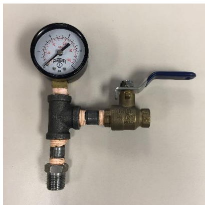
Figure 5. The Nitrogen Layup ASSY, used to fill the boiler with Nitrogen and monitor the pressure of the boiler.
