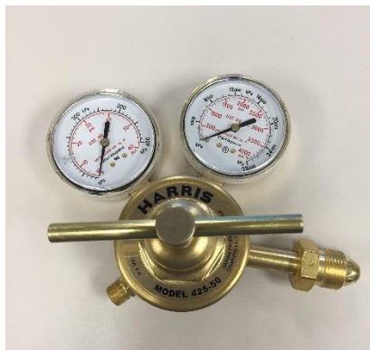
Figure 3. The Nitrogen regulator that controls the feed of Nitrogen into the boiler.
