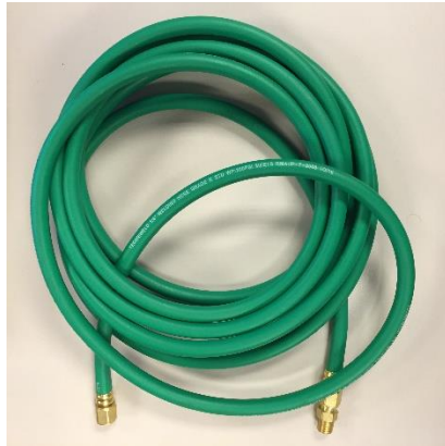
Figure 1. Hose to feed Nitrogen into the boiler.
