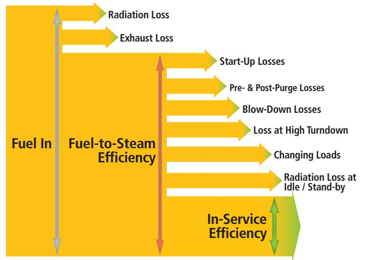
Miura's On-Demand boiler technology is engineered with the full spectrum of operating losses in mind with specific design features that address each to provide superior energy management capability and industry-leading In-Service Efficiency.
